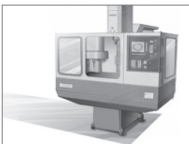
2 The CAD/CAM drawing is used to program the CNC machine.
