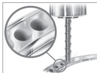
3 The CNC machine first mills the cavities into the metal part.
