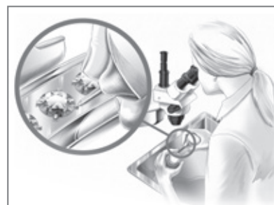
6 The manual beading and polishing of the prongs is often done under a microscope.
